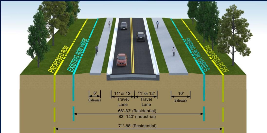
Build Alternative – One lane in each direction with curb and gutter on the outside. A six-foot sidewalk on the north side and a ten-foot sidewalk/shared use path on the south side. From CCNW to Mission Rd, travel lanes will be 12-foot wide. From Mission Rd to Ocala Rd, travel lanes will be 10 to 12-foot wide.
