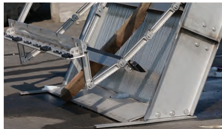
Factory demonstration of 4"x4" entering screen at bottom of channel.
