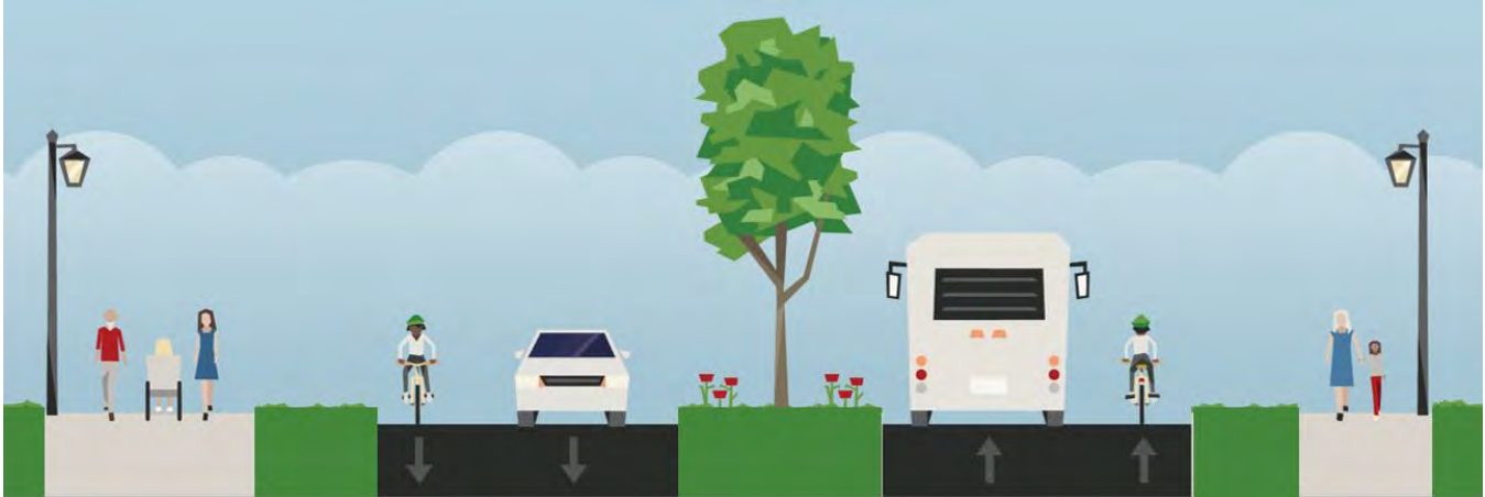
Figure 5. Conceptual Typical Section, New Roadway (Pottsdamer to Stuckey Avenue)
