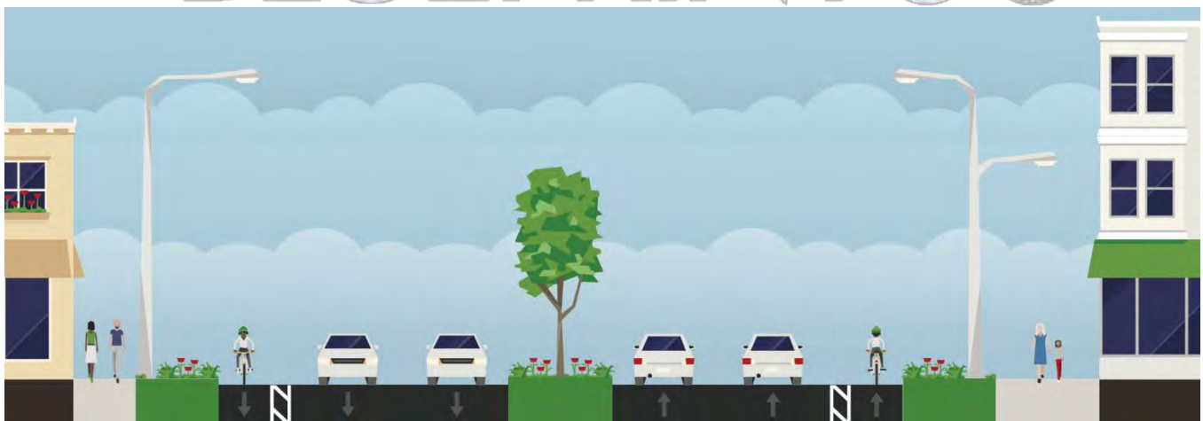
Figure 7. Conceptual Typical Section, North Lake Bradford Road
